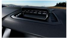
Ranger FX4 Max's upgraded 250A alternator is matched to an auxiliary switch pack allowing you to control your aftermarket accessories from the comfort of the driver's seat.
