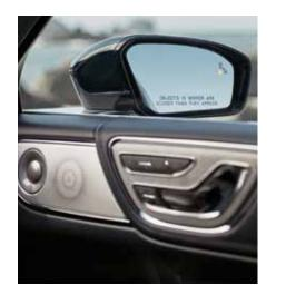
BLIS® (BLIND SPOT INFORMATION SYSTEM) WITH CROSS-TRAFFIC ALERT<sup>1,2</sup> – Some vehicles may be out of your line of sight, but they can be detected by this technology. It warns you if it detects a vehicle in your blind spots while driving forward, or approaching from the sides while in Reverse.
